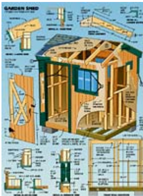
17 Position the door in its opening with a 1/4-in. space at the top and sides. Bore pilot holes for the hinge screws and secure the hinges.
